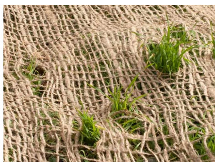
Figure 7: Jute mesh to be used for soil retention on the butterfly habitat roof garden
